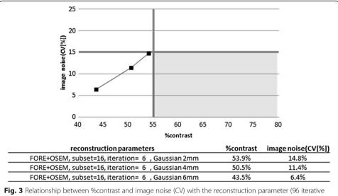
updates: iteration = 6 and subset = 16) and different post-filters (2, 4, and 6 mm FWHM Gaussian filter) for an old PET camera model measured with the phantoms under flutemetamol condition. Ninety-six iterative updates and other iterative updates (80 and 128, data not shown) did not satisfy the criteria (*shaded region*)
